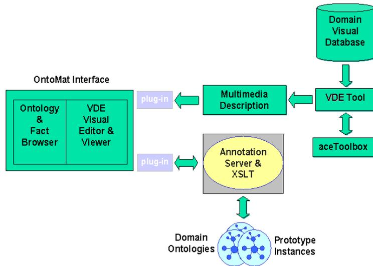
**Fig. 2.** OntoMat-Annotizer and VDE plug-in design architecture
